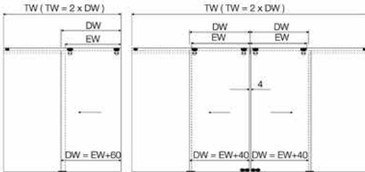
**Note : TW=Tube Length / DW=Door Width / EW=Entry Width
