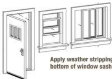
Apply weather stripping around door frame / stop.
