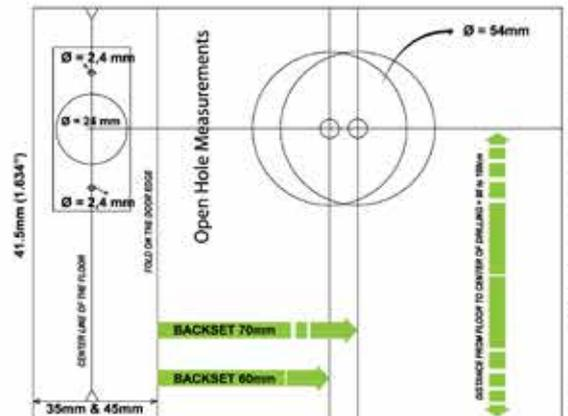
This lever will fit 35mm to 45mm door thickness
