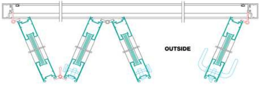
**HORIZONTAL SECTIONAL DETAIL ( WITH DOOR CLOSED )**
