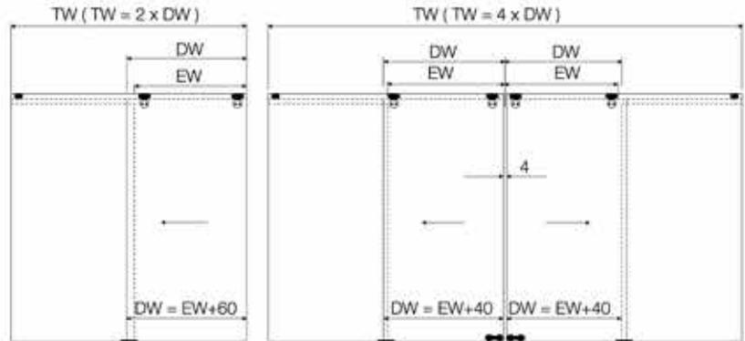
**Note : TW=Tube Length / DW=Door Width / EW=Entry Width**
